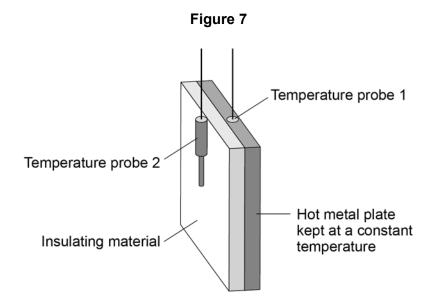
In the investigation different insulating materials were placed in contact with the hot metal plate.
